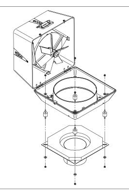
Fixate the flange to the chimney fan with the use of the vibration dampers supplied with the flange.
