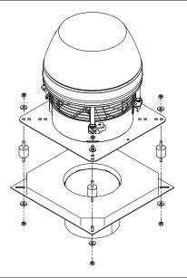
4 Fixate the flange to the chimney fan with the use of the vibration dampers supplied with the flange.
